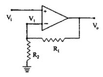
output resistance and a voltage gain A<sub>v</sub>. For the given circuit, find the gain with feedback (A<sub>vf</sub>):
