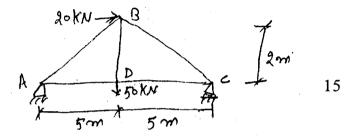
9. Analyze the truss as shown in figure by method of tension coefficients and determine the forces in the members AB, AE, BE and BC.
