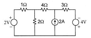
3. Derive the equation for star delta transformation. Find the value of current flowing through 2 ohm current in the given network by using star delta transformation.
